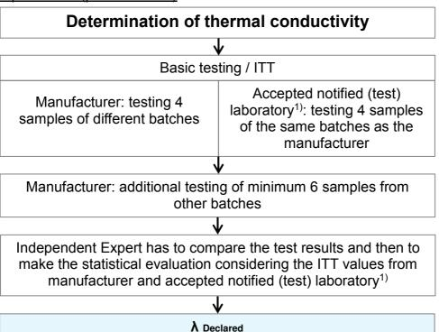
Accepted by PPA-Europe for thermal conductivity testing. As there are no notified bodies for thermal characteristics in case of EN 14509, the tests can be performed by notified bodies for testing the thermal conductivity of PU according to EN 13165, of MW according to EN 13162, of EPS according to EN 13163 or of XPS according to EN 13164, from the list of third parties accepted by PPA-Europe for thermal conductivity testing.
