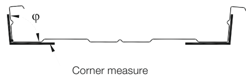
Figure 3.26: Measurement of corner angle flange/web
